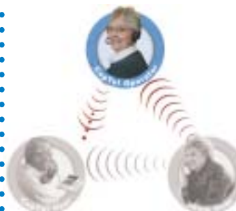
CapTel operator captions/transcribes Voice User's message into text by using voice-recognition technology.
