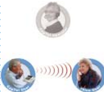
As CapTel User dials, the phone automatically connects to a captioning service. CapTel User talks directly to Voice User.
