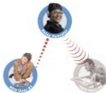
HCO User #1 types the conversation to relay operator. Relay operator voices the typed message by HCO User #1 to HCO User #2.
